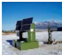
Solar Powered Chem Injection Pump
